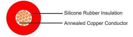
**Conductor:** Annealed copper conductor, class 5. **Insulation:** Silicone rubber.
