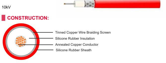
**Conductor:** Annealed copper conductor, class 5. **Insulation:** Silicone rubber. **Screen:** Tinned copper wire braiding. **Sheath:** Silicone rubber.
